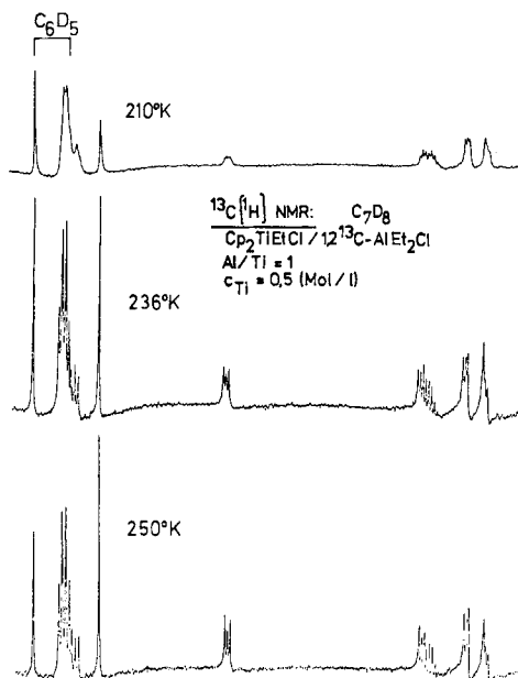
Fig. 10. ^{13}\text{C} -NMR spectrum of a mixture of \text{Cp}_2\text{TiEtCl}/\text{AlEt}_2\text{Cl} in \text{C}_6\text{D}_5\text{CD}_3 with 1,2- ^{13}\text{C} -enriched Al-alkyl. Ratio Al/Ti = 1; [\text{Cp}_2\text{TiEtCl}] = 0.5 mole/l.
